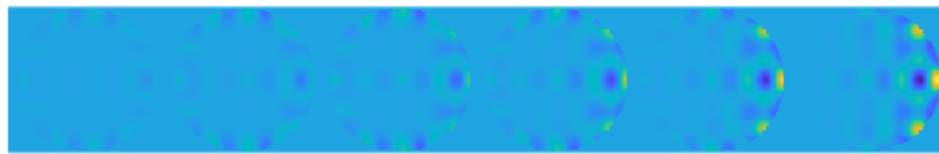
Figure 3-2: Phases resulting from increasingly large horizontal shifts of the LODM with P-Zernike mode 44 on the CalDM.
