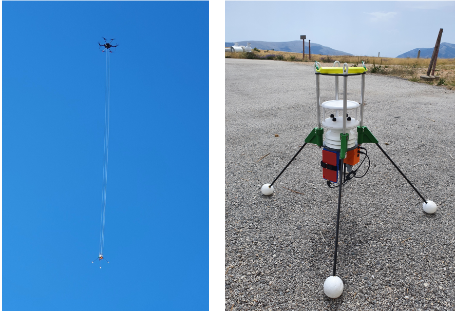
Figure 8: Picture of a drone flight (left) and of the instrumented nacelle (right). For more details see Ref. [15].
