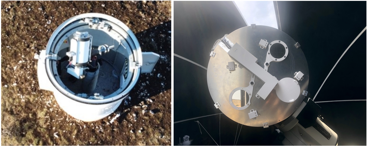
Figure 3. Left: the GMT instrument inside its 2.3m AllSky Baader dome. Right: The pupil mask and the optical device of the GMT instrument.
