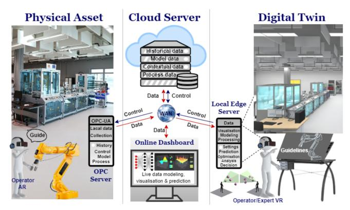
FIGURE 1. Digital Twin with XR in Edge/Cloud platform.
