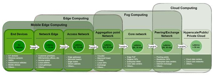
FIGURE 8. Network latency levels depending on the architecture and location.
