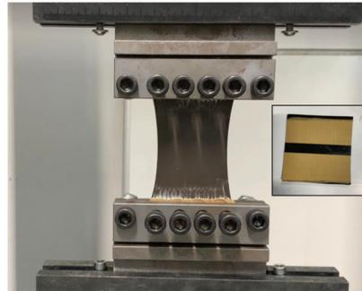
**Figure 2.** Pure shear specimen and test set-up.
