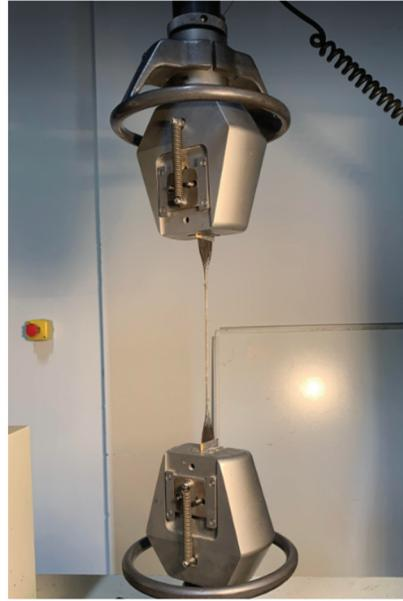
**Figure 1.** Uniaxial tensile test on a PR 1782 C2 dumbbell specimen.
