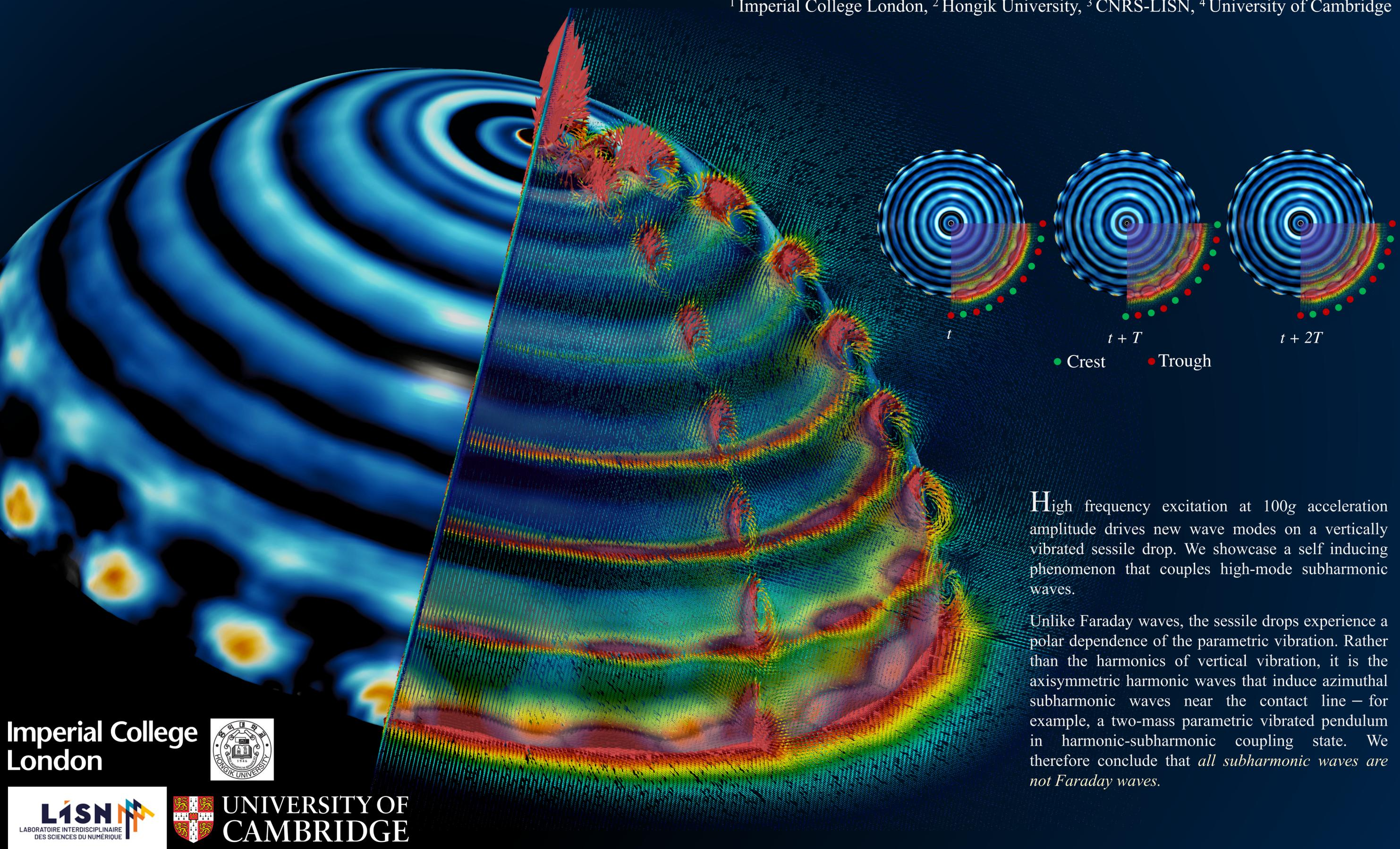
High frequency excitation at 100g acceleration amplitude drives new wave modes on a vertically vibrated sessile drop. We showcase a self inducing phenomenon that couples high-mode subharmonic waves.
