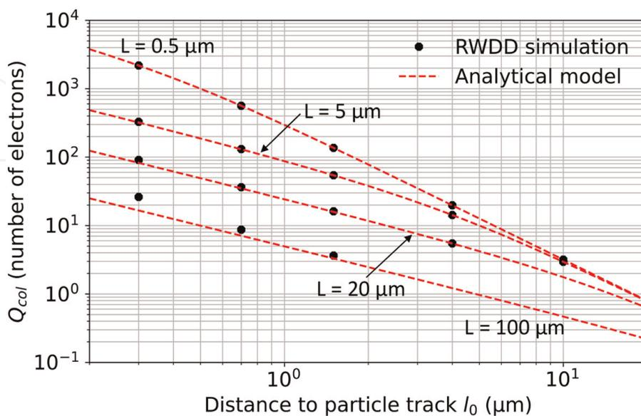
**Figure 7.** Collected charge versus the distance  $\ell_0$  from the collecting contact to the particle track of length  $L$  (see **Figure 5**). The collected charge is analytically calculated using Eq. (14) and numerically computed using the Monte Carlo RWDD simulation code.
