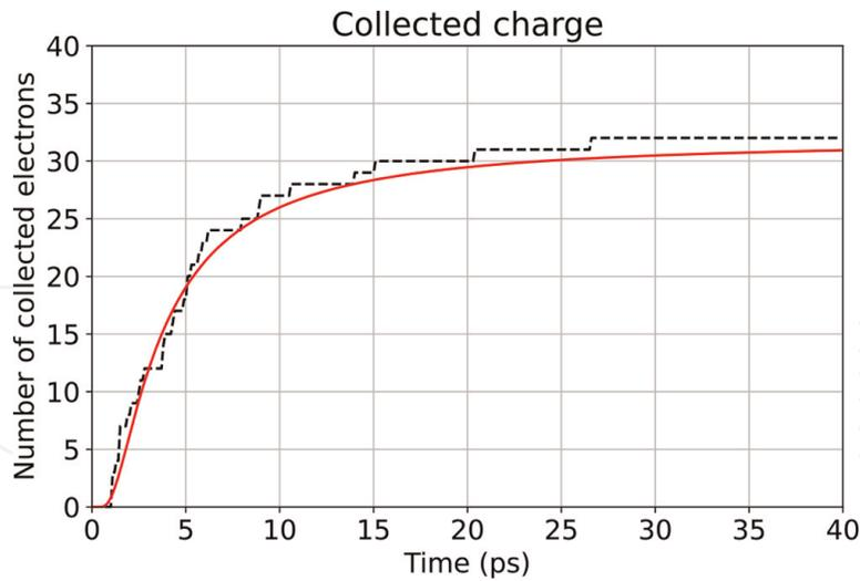
**Figure 4.** Time evolution of the charge collected by a small contact ( $A_C = 0.2 \times 0.2 \mu\text{m}^2$ ) located at  $1 \mu\text{m}$  from the initial deposition of 10,000 electrons (see **Figure 3**) analytically predicted by Eq. (8) and numerically computed using the Monte Carlo RWDD simulation code.
