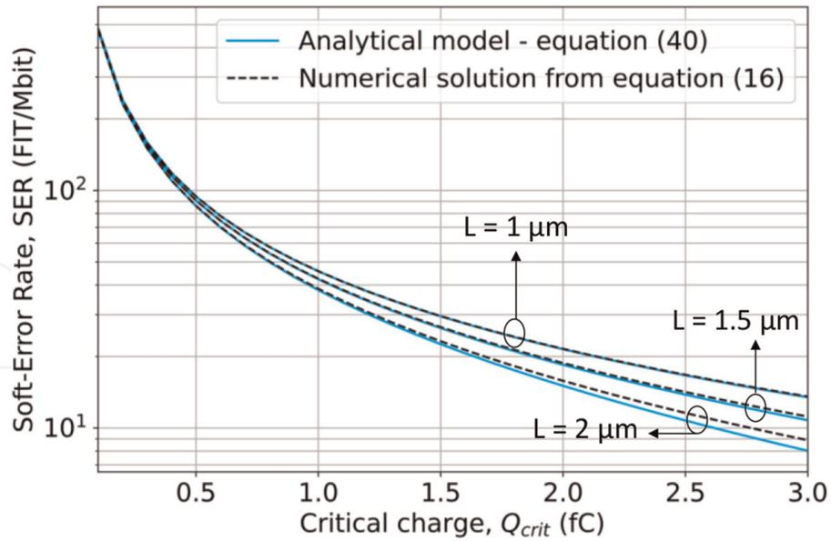
**Figure 9.** Soft-error rate as a function of the critical charge calculated from the analytical model of Eq. (40) and from the numerical solving of Eq. (16). Simulation parameters are as follows:  $A_C = 0.1 \mu\text{m}^2$ ,  $N = 1.38 \times 10^6$ ,  $D = 61 \text{ cm}^2 \text{ s}^{-1}$ , and  $F = 10^{-3} \text{ cm}^{-2} \text{ h}^{-1}$ .
