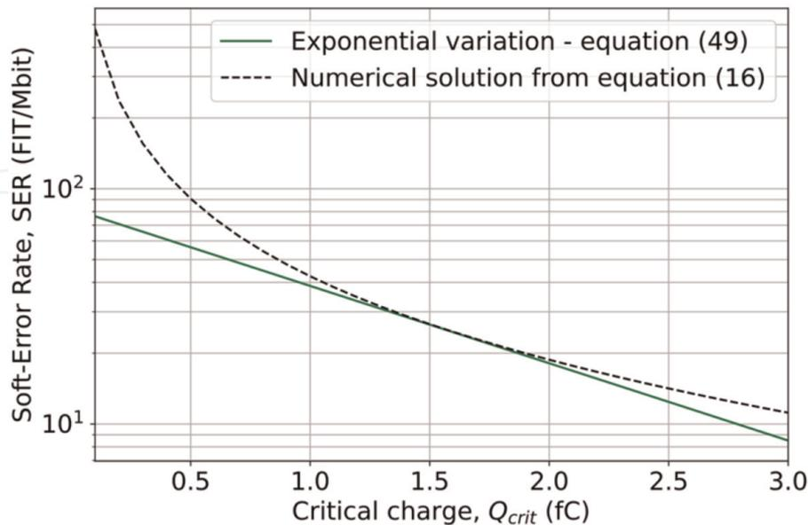
**Figure 10.** Soft-error rate as a function of the critical charge calculated from the analytical model of Eq. (49) and from the numerical solving of Eq. (16). Simulation parameters are as follows:  $A_C = 0.1 \mu\text{m}^2$ ,  $L = 1.5 \mu\text{m}$ ,  $N = 1.38 \times 10^6$ ,  $D = 61 \text{ cm}^2 \text{ s}^{-1}$ ,  $F = 10^{-3} \text{ cm}^{-2} \text{ h}^{-1}$ , and  $v_{COL} = 4.6 \times 10^5 \text{ cm s}^{-1}$  (in Eq. (49)).
