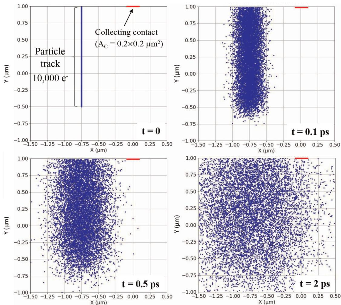
**Figure 6.** Distributions of charges in a vertical section along the x-y plane ( $z = 0$ ) at  $t = 0, 0.1, 0.5,$  and  $2$  ps after the deposition of 10,000 electrons along a  $1.5\text{-}\mu\text{m}$  length track located at  $0.75\text{ }\mu\text{m}$  from the contact. Other simulation parameters are the same as reported in the caption of Figure 3.
