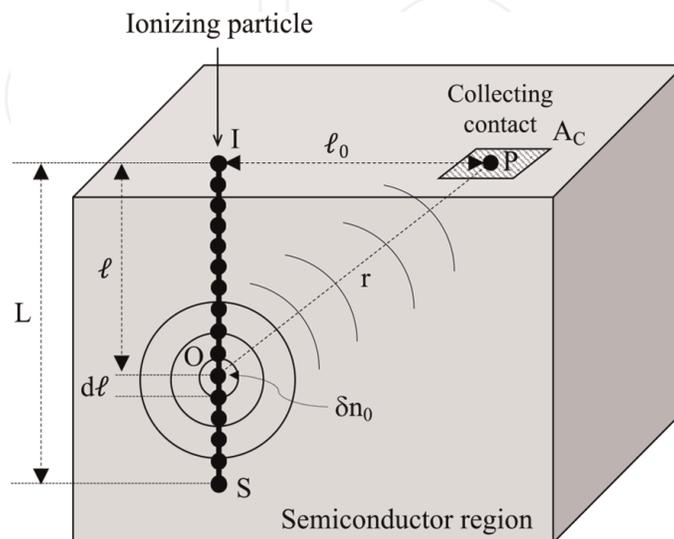
**Figure 5.** Schematic representation of a particle impact in the semiconductor region of a circuit. The particle track is treated as a set of point charges  $\delta n_0$  uniformly distributed along a straight segment of length  $L$ .
