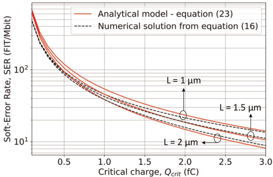
**Figure 8.** Soft-error rate as a function of the critical charge calculated from the analytical model of Eq. (23) and from the numerical solving of Eq. (16). Simulation parameters are as follows:  $A_C = 0.1 \mu\text{m}^2$ ,  $N = 1.38 \times 10^6$ ,  $D = 61 \text{ cm}^2 \text{ s}^{-1}$ , and  $F = 10^{-3} \text{ cm}^{-2} \text{ h}^{-1}$ .
