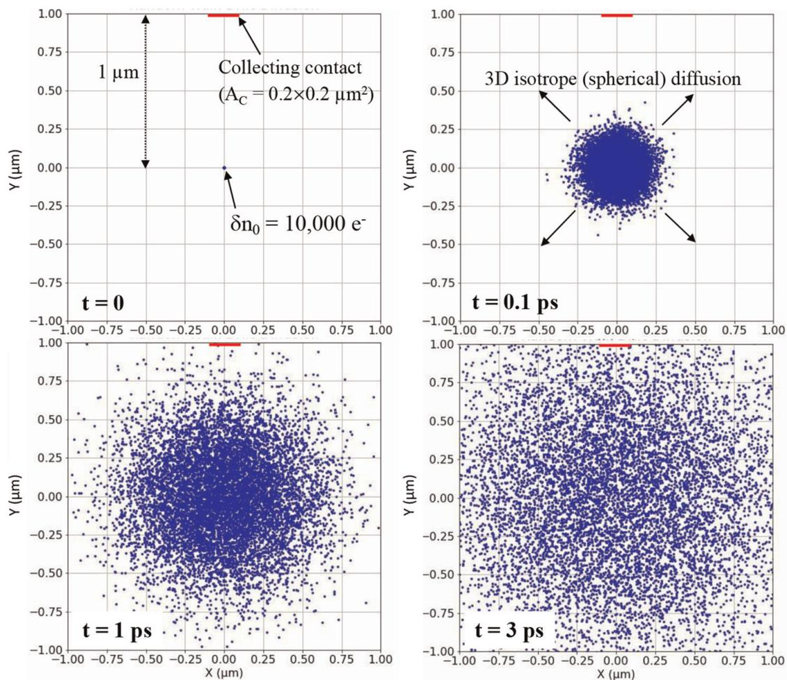
**Figure 3.** Distributions of charges in a vertical section along the  $x$ - $y$  plane ( $z = 0$ ) at  $t = 0, 0.1, 1$  and  $3 \text{ ps}$  after the deposition of 10,000 electrons at position  $(0, 0, 0)$ . Charges are transported following Eq. (10) with  $D^* = 533 \text{ cm}^2/\text{s}$ ,  $\Delta t = 0.1 \text{ ps}$ , and  $E_0 = 0$  (pure diffusion law). The surface of the collecting contact is in the  $x$ - $z$  plane, perpendicular to the figure.
