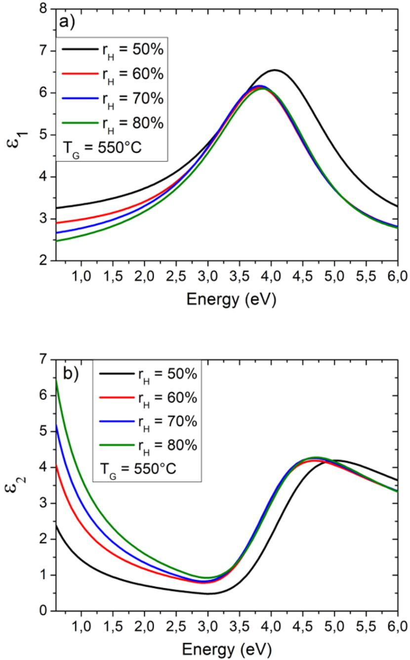
Figure 11: a) Evolution of the real part of the dielectric permittivity as a function of the energy for different values of  $r_H$  with  $T_G = 550^\circ\text{C}$ , b) Evolution of the imaginary part of the dielectric permittivity as a function of the energy for different values of  $r_H$  with  $T_G = 550^\circ\text{C}$ .
