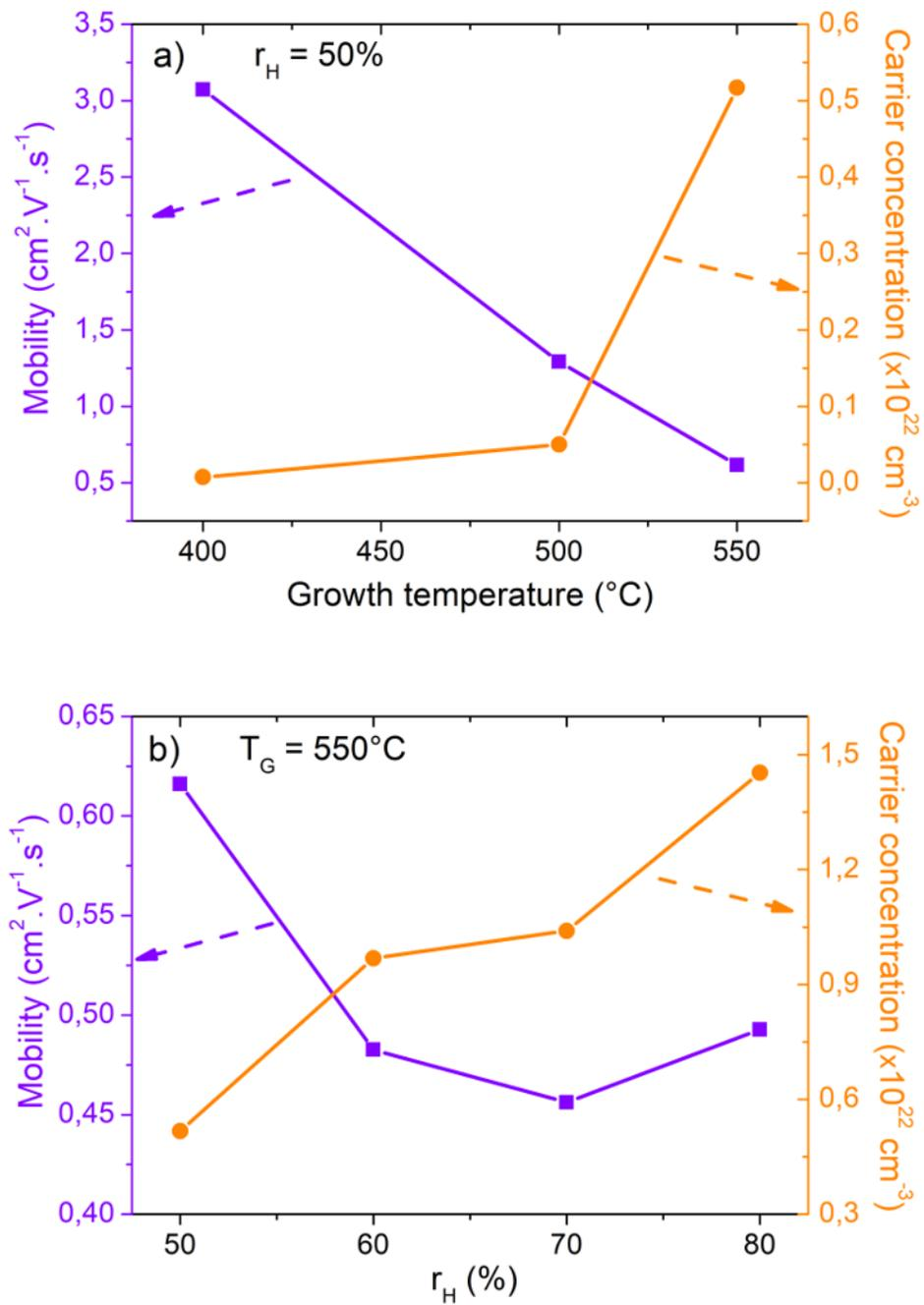
Figure 8: Transport properties at 300K. a) carrier concentration evolution at room temperature for different values of  $T_G$  and  $r_H$ , b) carrier mobility at room temperature for different values  $T_G$  and  $r_H$
