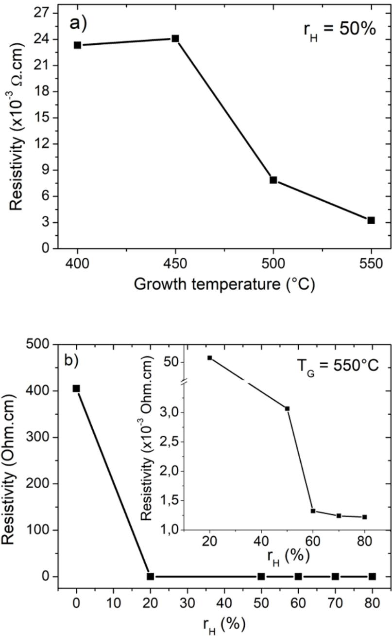
Figure 6: Electrical resistivities at room temperature obtained by the 4 probe method. a) for different values of  $T_G$  with  $r_H = 50\%$ , b) for different values of  $r_H$  with  $T_G = 550^{\circ}\text{C}$ .
