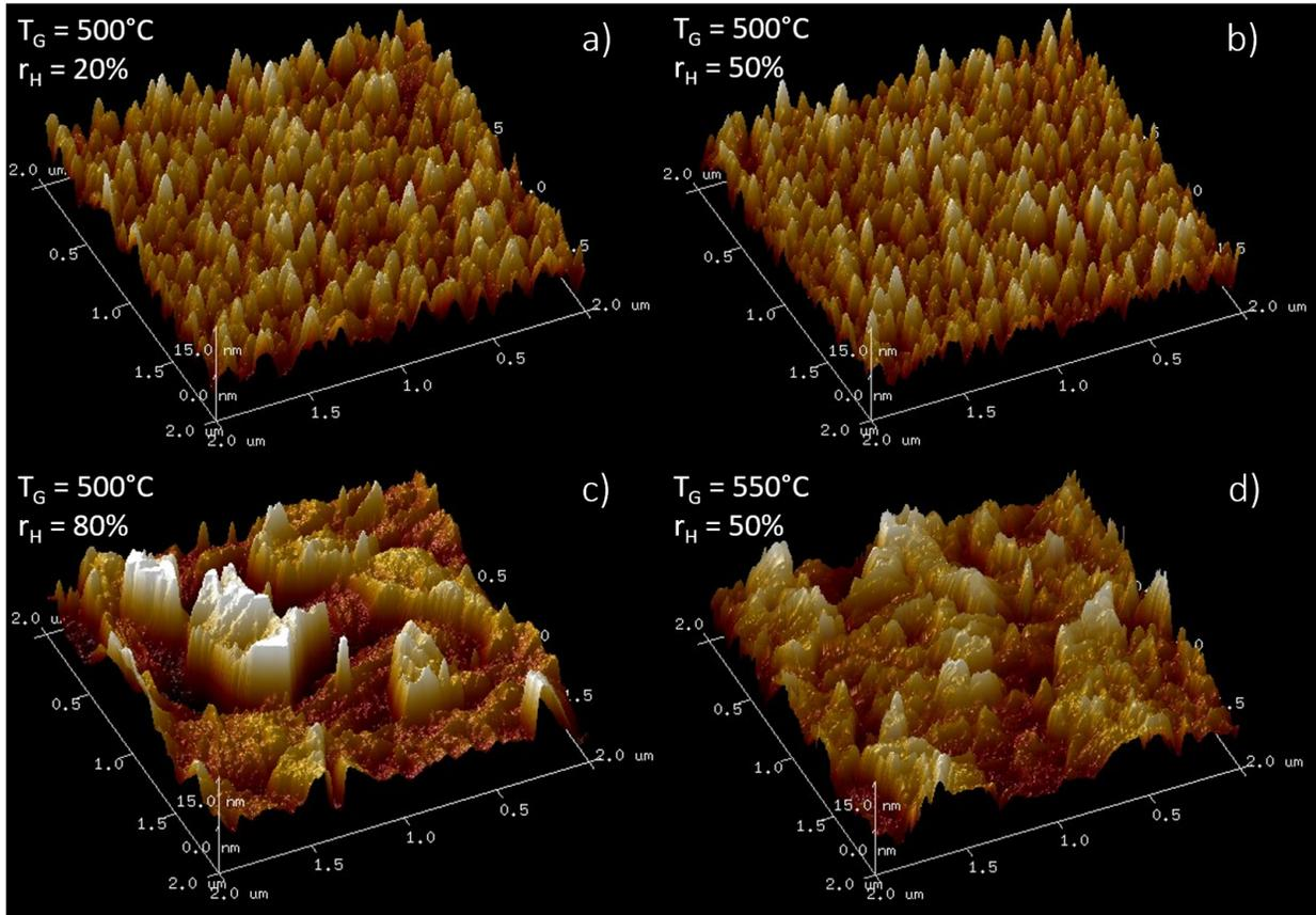
Figure 4: AFM images of the films obtained by sputtering of  $\text{Sr}_2\text{V}_2\text{O}_7$  target on Si substrates and anatase  $\text{TiO}_2$  seed layer. a) for  $T_G = 500^\circ\text{C}$  and  $r_H = 20\%$ , b) for  $T_G = 500^\circ\text{C}$  and  $r_H = 50\%$ , c) for  $T_G = 500^\circ\text{C}$  and  $r_H = 80\%$ , d) for  $T_G = 550^\circ\text{C}$  and  $r_H = 50\%$ . AFM images are  $2\ \mu\text{m} \times 2\ \mu\text{m}$
