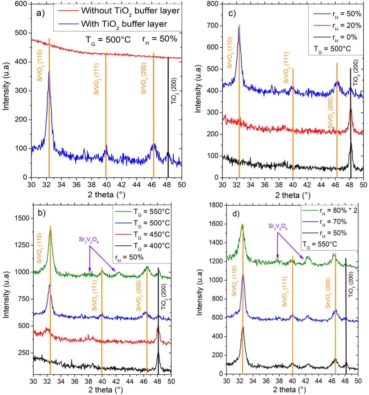
Figure 1: GIXRD patterns of thin film grown with sputtering of  $\text{Sr}_2\text{V}_2\text{O}_7$  target a) with and without a  $\text{TiO}_2$  seed layer b) for different values  $T_G$  and  $r_H = 50\%$ , c) for different values of  $r_H$  and  $T_G = 500^\circ\text{C}$ , d) for different values of  $r_H$  and  $T_G = 550^\circ\text{C}$ .
