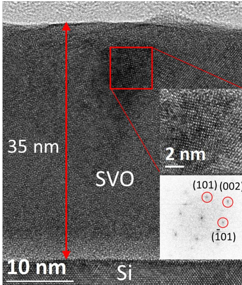
Figure 2: Typical HRTEM image of a SrVO<sub>3</sub> film grown directly on a (100) Si substrate, at 500°C with  $r_H = 50\%$ . SrVO<sub>3</sub> small grains are clearly visible in the film.
