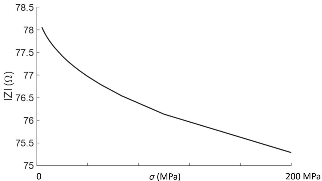
Fig. 6 – Illustration of a uniaxial homogeneous stress influence on the impedance modulus of an eddy current sensor.
