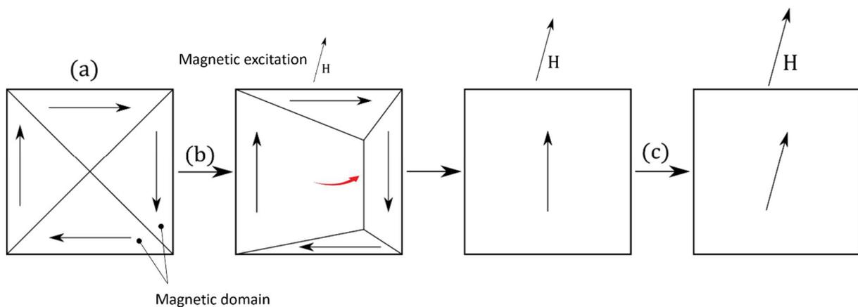
Fig. 4 – Schematic illustration of the magnetization process. (a) Demagnetised state (b) Domain wall motion (c) Magnetisation rotation. In practice, the two mechanisms can occur simultaneously.
