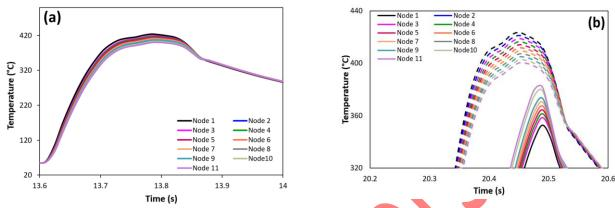
Figure 11 – Zoom on the temperature profiles from Figure 10 to observe in (a) thermal gradients through the thickness of ply 3 during its deposition & (b) thermal gradient through the thickness of ply 3 (continuous lines) and ply 4 (dashed lines) during the deposition of ply 4 on top of ply 3.
