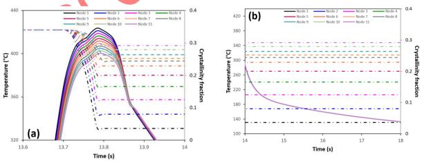
**Figure 12-**Evolution of the temperature and crystallinity fraction for the different nodes of Ply 3 during its deposition. Continuous lines (-) present the temperature while dashed lines (-.-) present the crystallinity.
