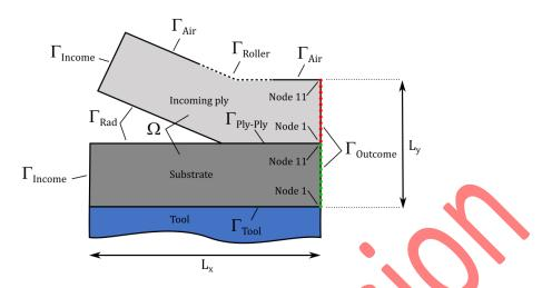
Figure 8 – Schematic presentation of the problem boundaries and nodes through the thickness of a ply.
