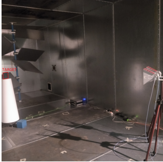
(a) Picture of the measurement set up in HH polarization in the RC
