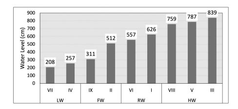
Medium water level at FIGURE 4 each mission; LW, low water; F, flushing; R, rising and HW, high water.
