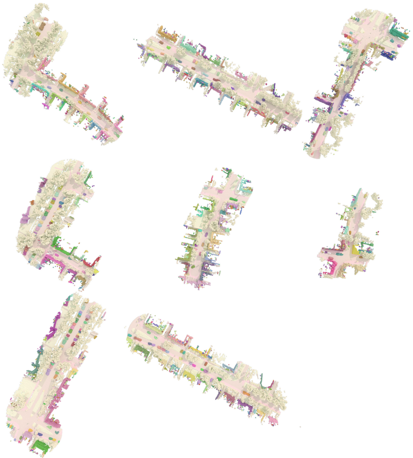
Figure A-6. Large-Scale Inference on KITTI-360. Largest scan that SuperCluster can segment in one inference on an A40 GPU: 7.5 tiles, 11.0M points, 414k superpoints, 602 target objects, and 1947 predicted objects. Inference takes 6.6 seconds.
