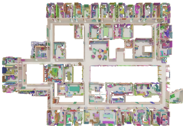
Figure 1. Large-Scale Panoptic Segmentation. We present the results of SuperCluster for the entire Area 5 of S3DIS [4] (ceiling removed for visualization) with 9.2M points (78M pre-subsampling) and 1863 true “things” objects. Our model can process such large scan in one inference on a single V100-32GB GPU in 3.3 seconds and reach a state-of-the-art PQ of 50.1.
