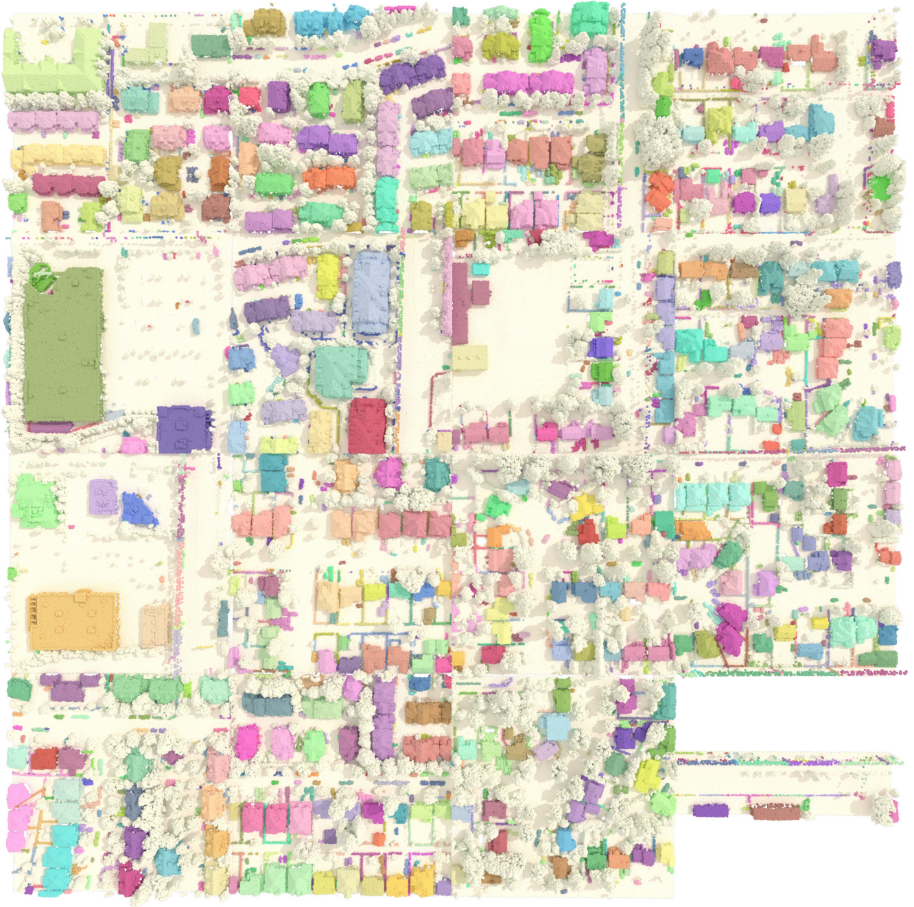
Figure A-5. Large-Scale Inference on DALES. Largest scan that SuperCluster can segment in one inference on an A40 GPU: 15.3 tiles, 7.8 km 2 , 18.0M points, 589k superpoints, 1727 target objects, and 1559 predicted objects. Inference takes 10.1 seconds.
