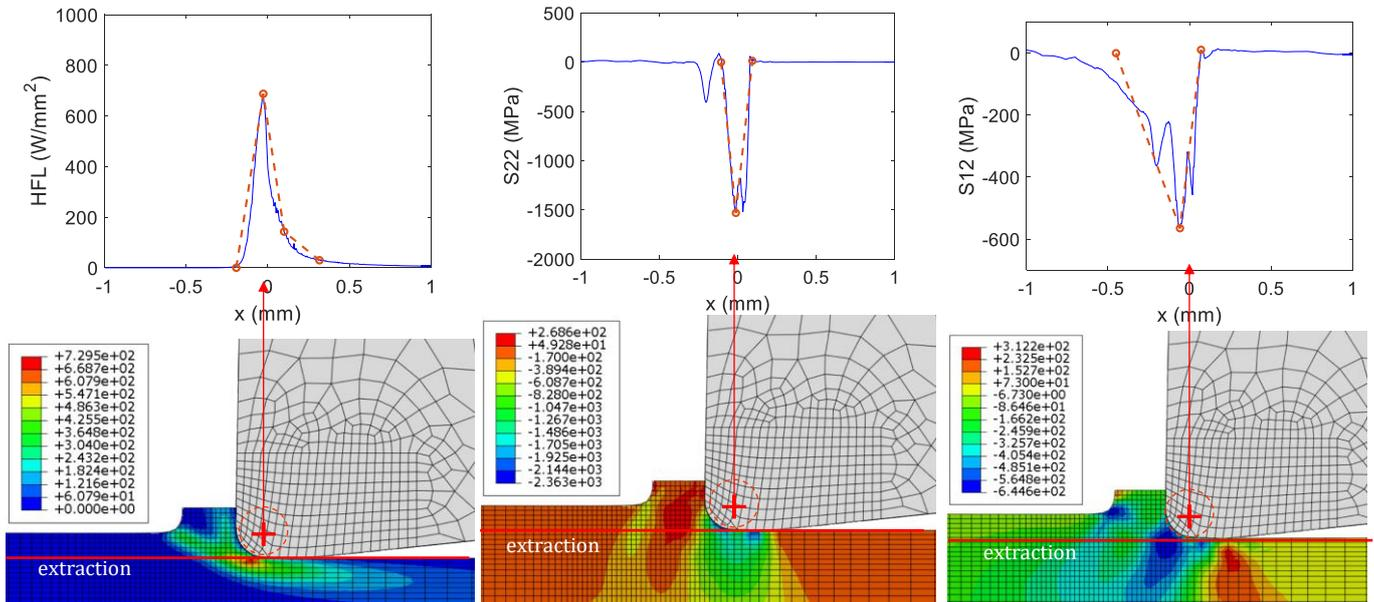
Figure 3 – Extractions of thermo-mechanical loadings (HFL, S22, S12) with  $h = 0.05$  mm and their approximations.
