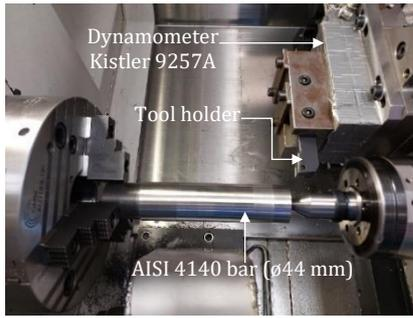
Figure 1 – Experimental setup for turning of AISI 4140 steel.
