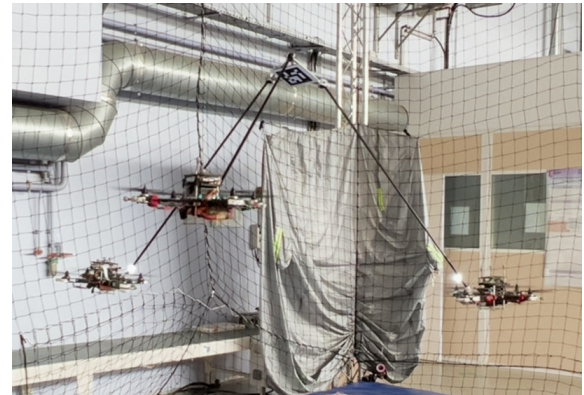
Figure 1: A flying parallel robot composed of a moving platform supported by three quadrotors with rigid legs.
