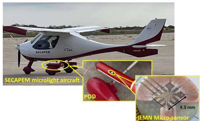
Fig. 4. Set up of the microlight aircraft flight experiments: photograph of the Flight Design CTSW microlight aircraft with a zoom on the PODs and on the calorimetric micro-sensor chip
