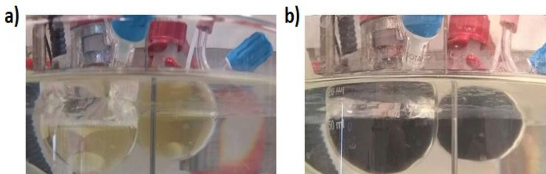
**S8:** Aqueous dispersion formation of the ion-sensitive PEDOT based ink: a) Before the addition of the oxidants, brownish polyelectrolyte solution; b) After addition of the oxidants, formation of the PEDOT based ink.
