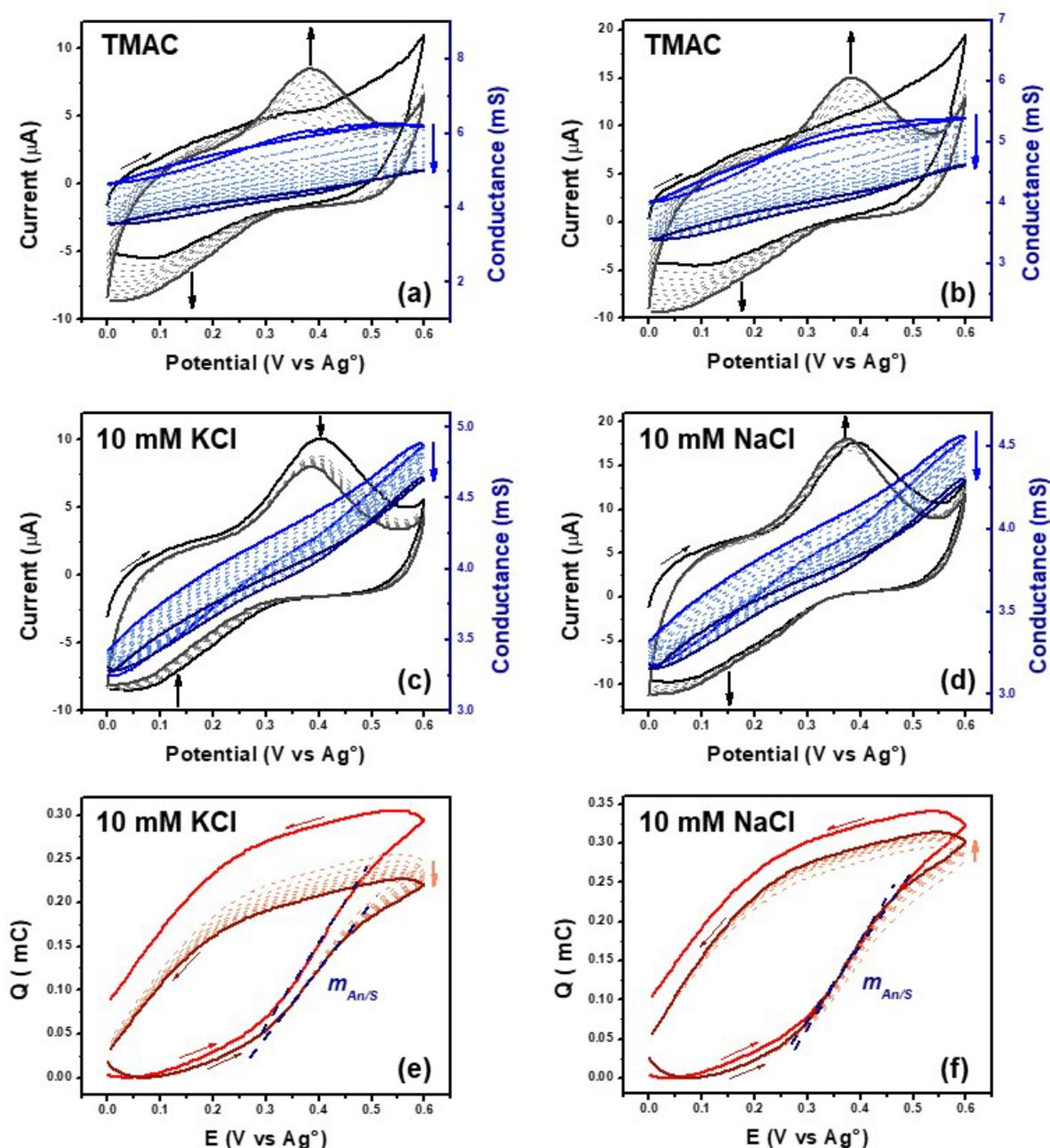
**Figure 2.** Simultaneous electrochemical (left axis black curves) and conductance (right axis blue curves) study of drop casted PEDOT/ P(STFSI<sub>85</sub>-co-S18cr<sub>615</sub>) films in a 0.1 M TMAC aqueous solution using  $E_{\lambda} = 0.6$  V vs Ag<sup>0</sup>, 10 cycles,  $\nu = 10$  mV s<sup>-1</sup> and  $\Delta V$  on the WE = 10 mV, WE = Pt IDMAE, CE = Pt foil, in the absence (a and b) and in the presence of (c) 10 mM
