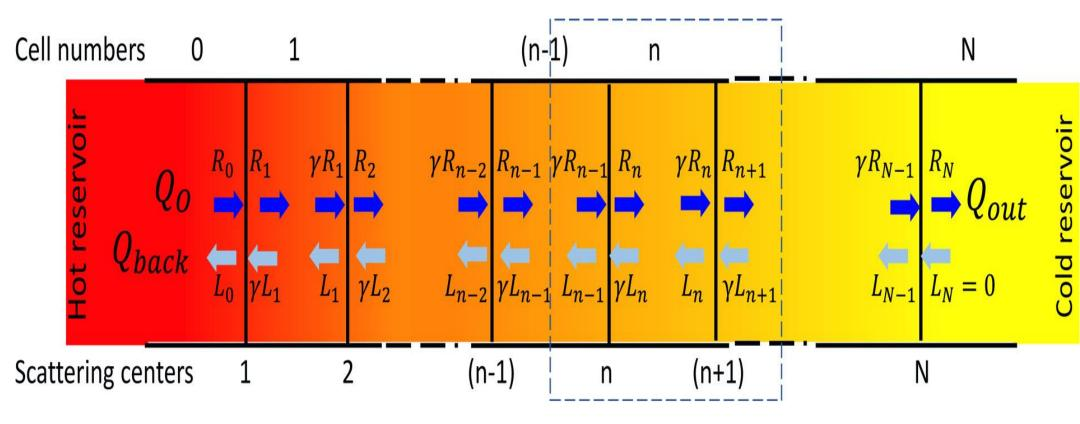
Flux flow balance between  $n^{\text{th}}$  and  $(n^{\text{th}}+1)$  cells :
