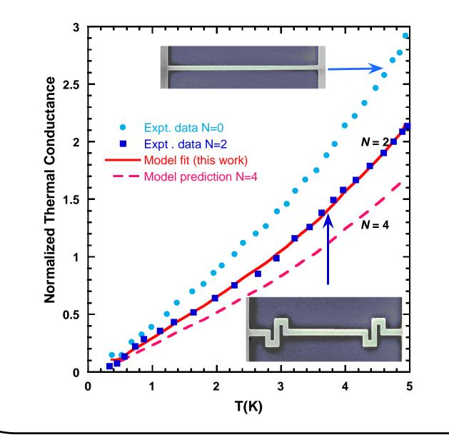
Experimental data of thermal conductance of Si nanowires normalized w. r. t. 4 quanta of thermal conductance : O. Bourgeois *et al*. C. R. Phys. 17, 1154 (2016) Copyright 2016, Elsevier [4]
