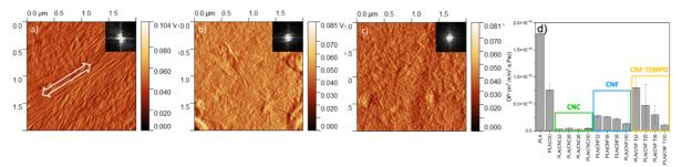
Figure 1 : AFM images of the sample surfaces coated with 10 deposits of CNC (a), CNF (b) and CNF TEMPO (c), and dry Oxygen permeabilities of uncoated and coated-PLA (d).
