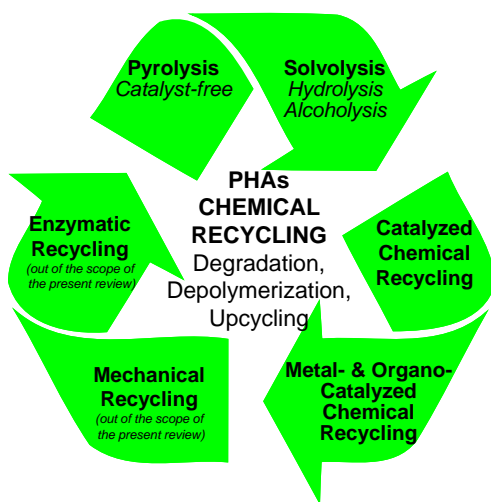
Fig. 2. Overview of the chemical recycling of PHAs.
