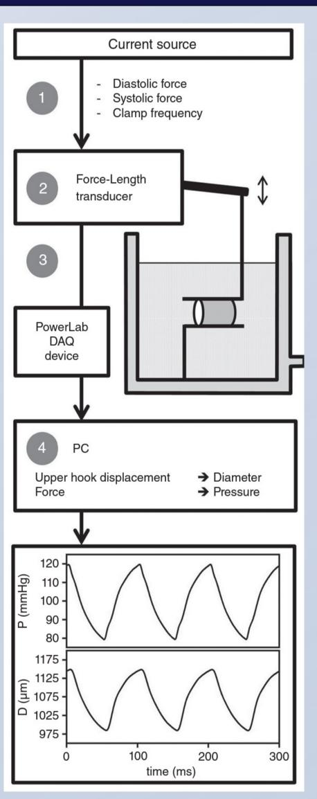
**Figure 1**. Schematic diagram of the ROTSAC.
