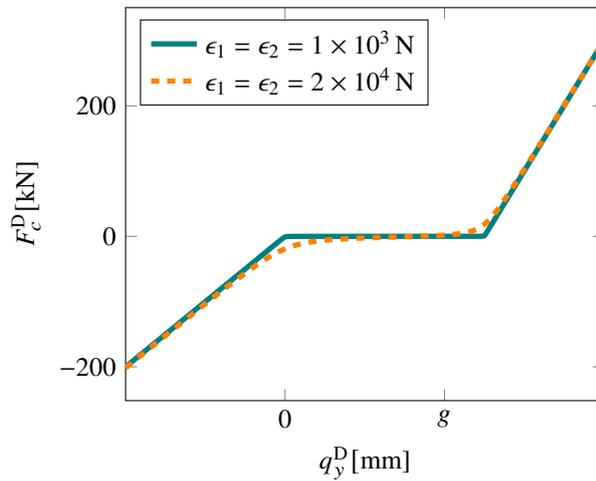
Figure 19: Representation of the contact force for  $k_1 = 5 \times 10^7 \text{ N m}^{-1}$ ,  $k_2 = 1 \times 10^8 \text{ N m}^{-1}$ ,  $g = 4 \text{ mm}$  and different values of the smoothing parameters.
