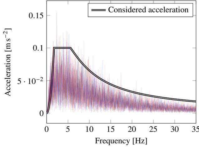
Figure 20: Base motion acceleration spectrum.
