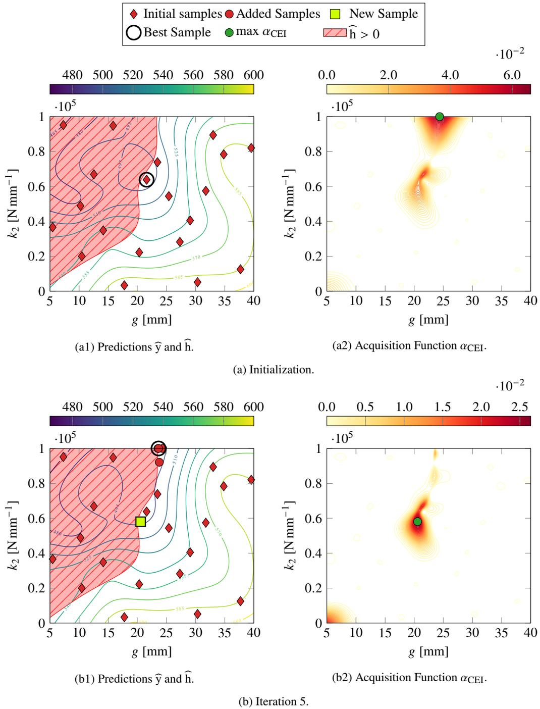
Figure 22: Constrained optimization process for 20 initial samples. Contour lines represent the objective function (in  $\text{mm s}^{-1}$ ), the red hatched area is the predicted unfeasible domain ( $h > 0$ ) and the black circle indicates the best feasible sampled parameters set.
