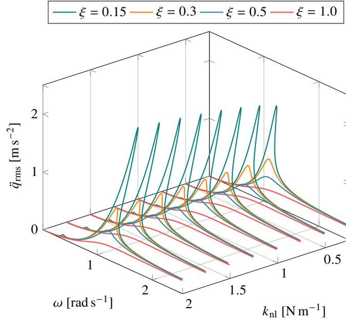
Figure 11: Frequency responses for a few pairs of values of  $\xi$  and  $k_{nl}$ .
