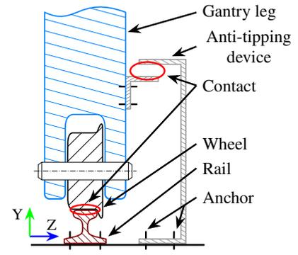
Figure 17: Illustration of an anti-tipping device.
