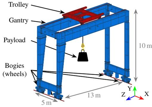
Figure 16: Model of the gantry crane.
