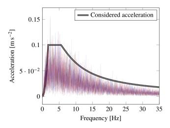
Figure 20: Base motion acceleration spectrum.
