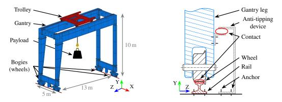
Figure 16: Model of the gantry crane.
