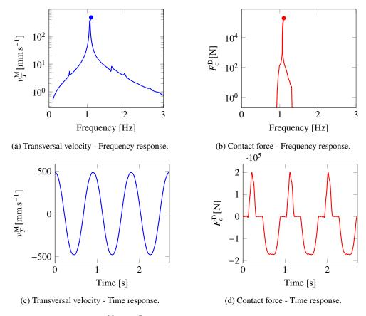
Figure 24: Frequency response of  $v_T^{\rm M}$  and  $F_c^{\rm D}$  as well as their time representations over 3 periods at their maximal value (excitation frequency of 1.11 Hz).
