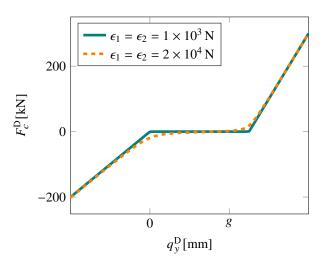
Figure 19: Representation of the contact force for  $k_1 = 5 \times 10^7 \,\mathrm{N}\,\mathrm{m}^{-1}$ ,  $k_2 = 1 \times 10^8 \,\mathrm{N}\,\mathrm{m}^{-1}$ ,  $g = 4 \,\mathrm{mm}$  and different values of the smoothing parameters.
