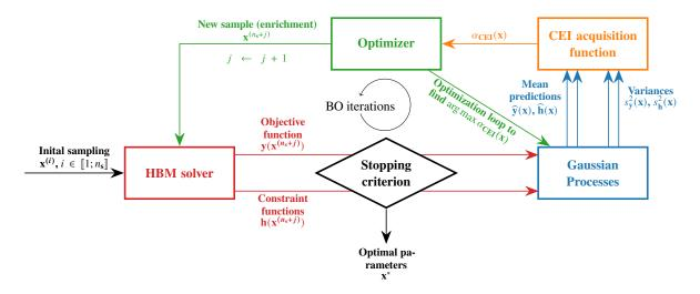
Figure 1: Workflow of the constrained optimization strategy.
