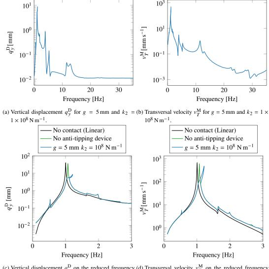
(c) Vertical displacement  $q_y^D$  on the reduced frequency (d) Transversal velocity  $v_T^M$  on the reduced frequency bandwidth for different configurations.
