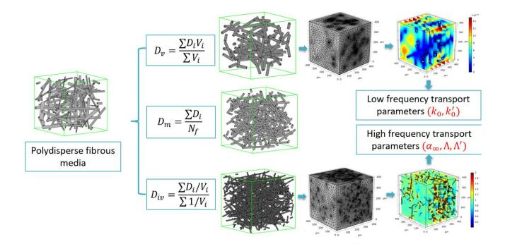
Figure 1: Illustration of the proposed methodology used to identify the microstructural descriptors  $D_v$  and  $D_{iv}$  enabling to predict the transport and sound absorbing properties of a polydisperse random fibrous media. Note that  $D_v$  is the volume weighted average diameter,  $D_{iv}$  is the inverse volume weighted average diameter, whereas  $D_m$  is the average diameter;  $V_i$  is the volume of the *i*<sup>th</sup> fiber and  $N_f$  corresponds to the number of fibers.
