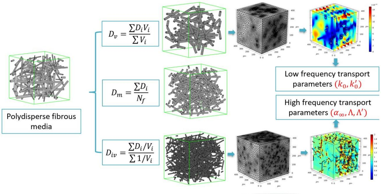
Figure 1: Illustration of the proposed methodology used to identify the microstructural descriptors  $D_v$  and  $D_{iv}$  enabling to predict the transport and sound absorbing properties of a polydisperse random fibrous media. Note that  $D_v$  is the volume weighted average diameter,  $D_{iv}$  is the inverse volume weighted average diameter, whereas  $D_m$  is the average diameter;  $V_i$  is the volume of the  $i^{\text{th}}$  fiber and  $N_f$  corresponds to the number of fibers.
