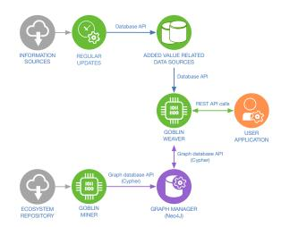
Figure 2: Architecture of the GOBLIN framework
