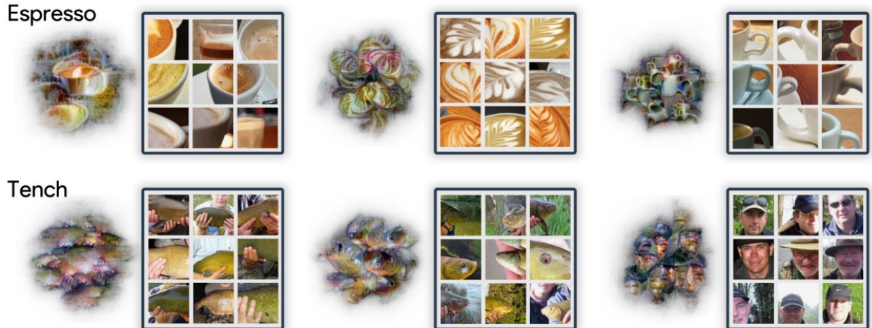
Figure 9 – Global explanation from CRAFT for two classes of ILSVRC2012 [9] for a pre-trained ResNet50V2 [22]. For each class, it shows crop images that activate the concept the most of the top 3 most important concepts. It also shows feature visualizations of the associated concepts.
