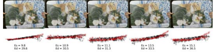
Fig. 9: Experiment with an almost stationary object. The first five images of the table mat sequence are used. The reconstruction of iso is shown in red. The ground truth is indicated with black. E_s represents the mean shape error (in degrees). E_d represents the mean depth error (in mm). The performance of iso is almost the same as infP on these five images.
