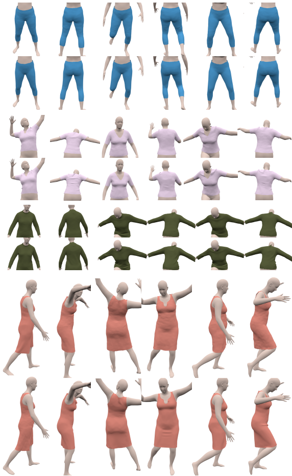
Fig. 11: GarNet-Local (top) vs PBS (bottom) results for several poses. Note how similar they are, even though the former were computed in approx. 70ms instead of 20s. Our method successfully predicts the overall shape and details with intermediate frequency.
