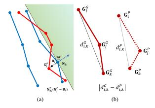
Fig. 6: Interpenetration and Bending loss terms. (a) The interpenetration term  $L_{pen}$  penalizes a garment vertex  $\mathbf{G}_{j}^{P}$  for being on the wrong side of the corresponding body point  $\mathbf{B}_{i}$ . (b) The bending term  $L_{bend}$  penalizes the distance between two neighbors of  $\mathbf{G}_{j}^{P}$  to differ from that in the ground truth.
