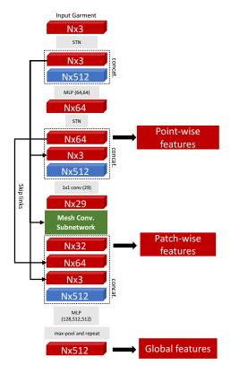
Fig. 3: **Garment branch of our network.** The grey boxes and the numbers in parenthesis denote network layers and their output channel dimensions. Red and blue ones represent garment and global body features, respectively. The green box is the mesh convolution subnetwork and depicted in more detail in Fig. 4. STN stands for a Spatial Transformer Network used in PointNet [43]. MLP blocks are shared by all N points.
