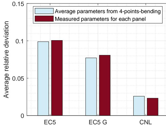
Figure 11. Average relative deviation from experimental values for Eurocode 5 with or without shear (EC5 G, EC5), and Non-Linear Criterion (NLC).
