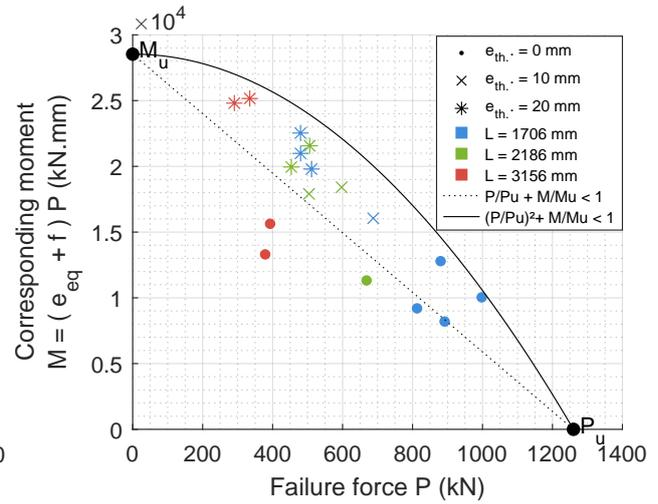
Figure 5. Interaction diagram without correction, Figure 6. Interaction diagram with corrected signal,  $M = (e_{eq} + f)P$
