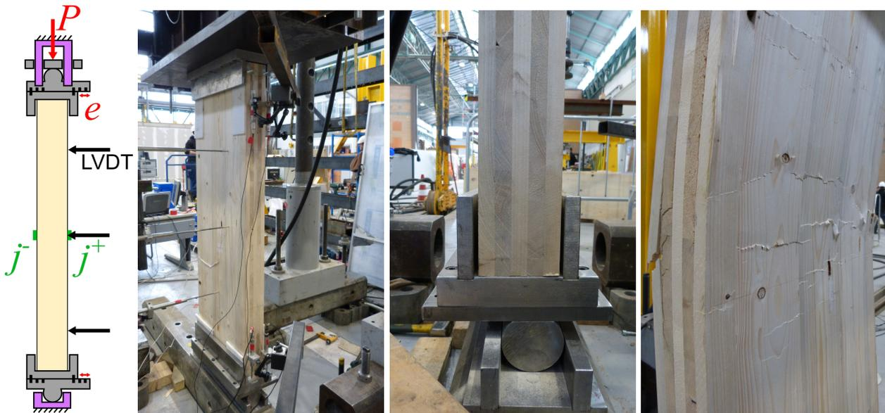
Figure 2. Typical buckling test
