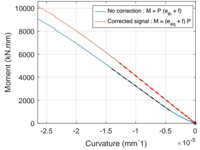
Figure 4. Moment before and after signal correction (Panel 24)
