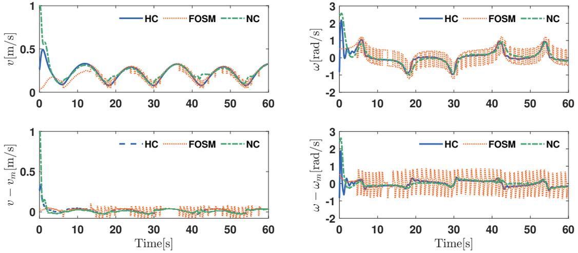
Fig. 4: Experimental Results for Control Signals. Signals  $v_m$  and  $\omega_m$  are from current measurements.
