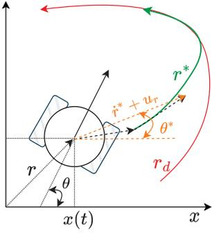
Fig. 1: Schematic Solution. This figure highlights that in the case of a large initial error, a nominal trajectory  $[r^*, \theta^*]$  may be employed to guide the system toward the desired trajectory  $[r_d, \theta_d]$ .
