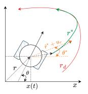
Fig. 1: Schematic Solution. This figure highlights that in the case of a large initial error, a nominal trajectory  $[r^*, \theta^*]$  may be employed to guide the system toward the desired trajectory  $[r_d, \theta_d]$ .
