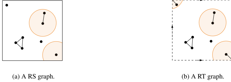
Figure 3: Showing the main difference between the RS and the RT graphs. In both cases, the nodes are connected if they are at a distance less than a radius r . In the RS graph the nodes are distributed on a square, hence the node on the bottom right and the node on the top left are not connected; on the torus, on the contrary, they are connected.
