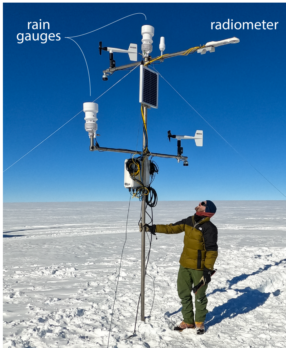
Figure S4. Newly-installed GEUS GC-Net AWS at South Dome. June 21, 2021 Photo J. Box.
