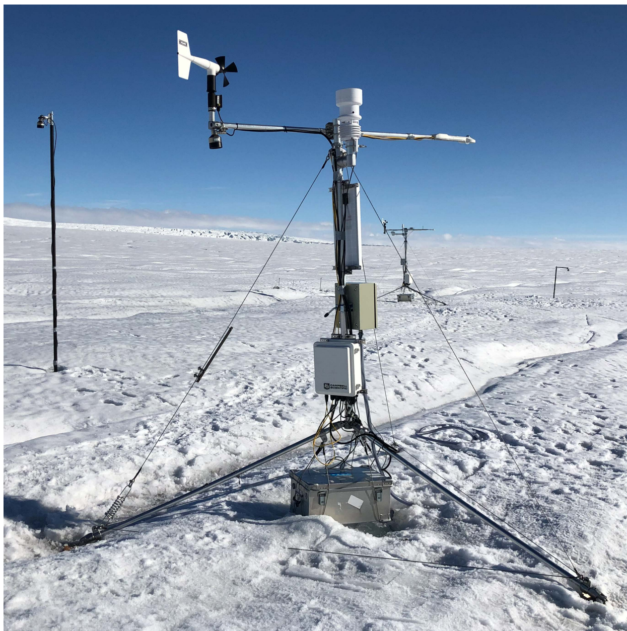
Figure S2. NUK_U PROMICE AWS with rain gauge (foreground) on 10 September, 2021_U and older PROMICE AWS version in background. Photo Jakob Jakpbsen.
