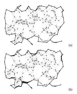
Figure 5: LPCN algorithm with (a) and without (b) intersections executed on a graph with 60 nodes.
