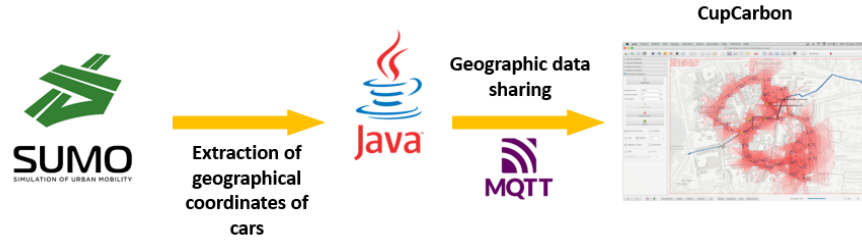
Fig. 1: Global process map of the developed application.
