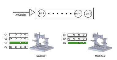
Fig. 1: RMS Modelling with RMT machines with differents configurations.
