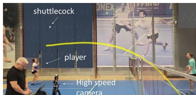
Figure 3. A high-speed camera captured videos of the trajectories of the shuttlecock at 3,700 fps on the badminton court, as players performed different cross-court slice shots.
