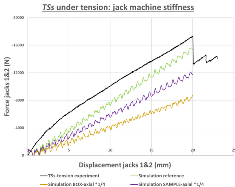
Figure 25. TSs sample under tension: effect of the variation of a few parameters on the machine jack stiffness and comparison with experiment.
