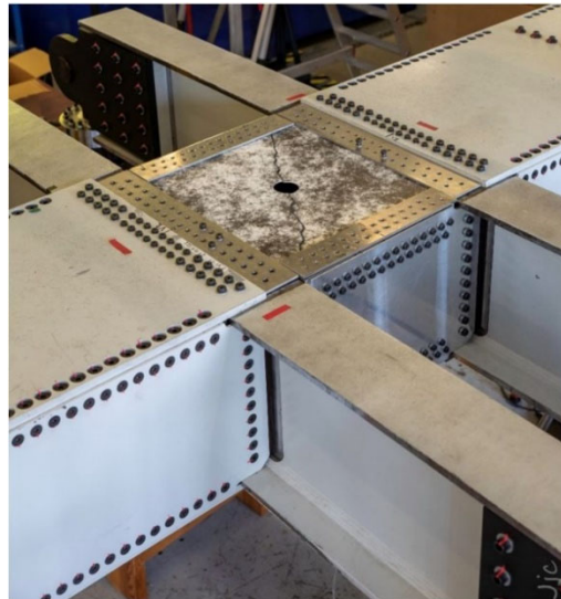
Figure 18. Picture showing the many bolts (black dots) composing the VERTEX test rig up to the sample, focusing on the central box (open-hole VERTEX sample, not presented here).
