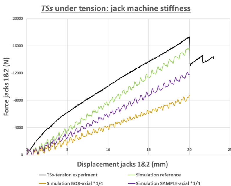
Figure 25. TSs sample under tension: effect of the variation of a few parameters on the machine jack stiffness and comparison with experiment.
