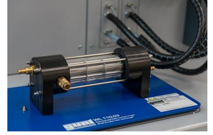
Shell and tubes micro heat exchanger
