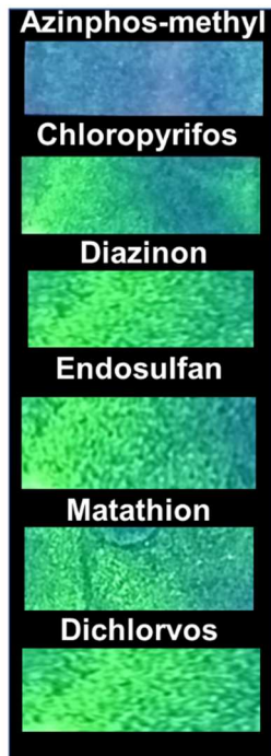
Figure S34. Colour of Tb-phen coated paper strips in presence of different pesticides (75 \mu M). Note: the green colour vanishes only in the presence of azinphos-methyl.
