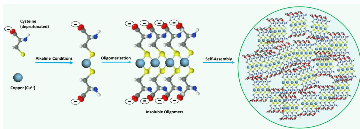
**Scheme 1.** Schematic representation of Cu-Cys self-assembled nanoparticles synthesis.
