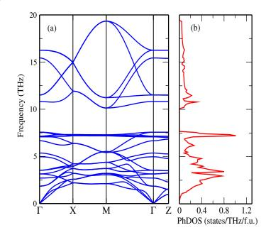
FIG. 5: (a) Phonon dispersion and (b) phonon density of states of ThCrAsN with G-AFM spin configuration.
