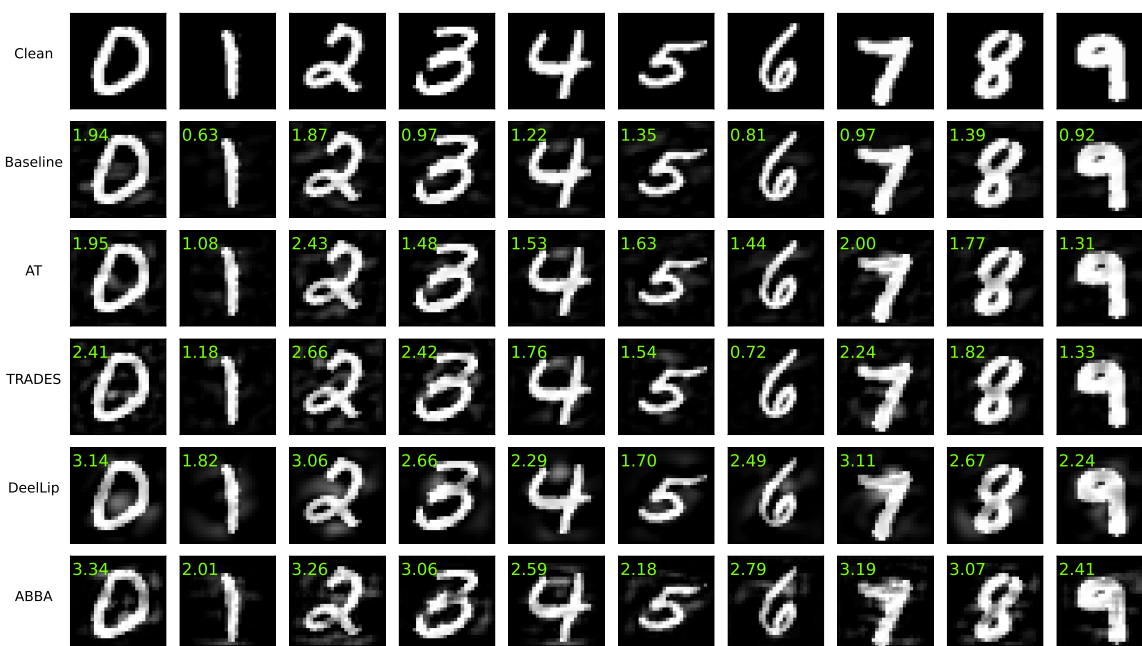
Figure SM2. Adversarial examples with DDN attack for Conv-Dense models, on MNIST dataset. \ell_2 perturbation magnitude is given in the top-left corner.
