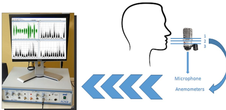
Fig. 2 Schematic representation of Experiment 2. Data were recorded simultaneously through built-in features of the EVA2 workstation: airflow velocity exhaled in three positions from the mouth were recorded by the three anemometers; wave signal and SPL intensity by a microphone
