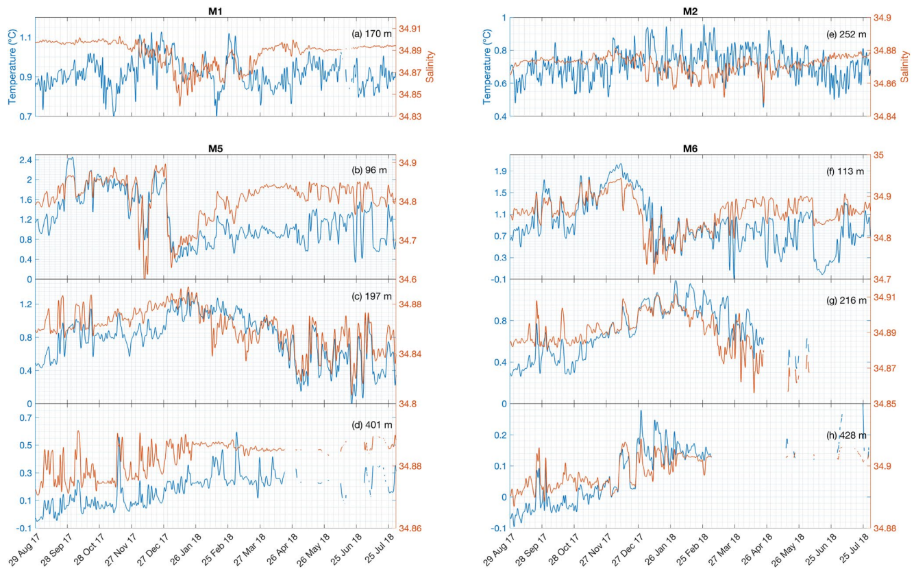
Figure 8. Time series of (blue) temperature and (orange) salinity recorded at (a) M1, (e) M2, (b–d) M5 and (f–h) M6. The depth of the sensor is displayed in the right upper corner.
