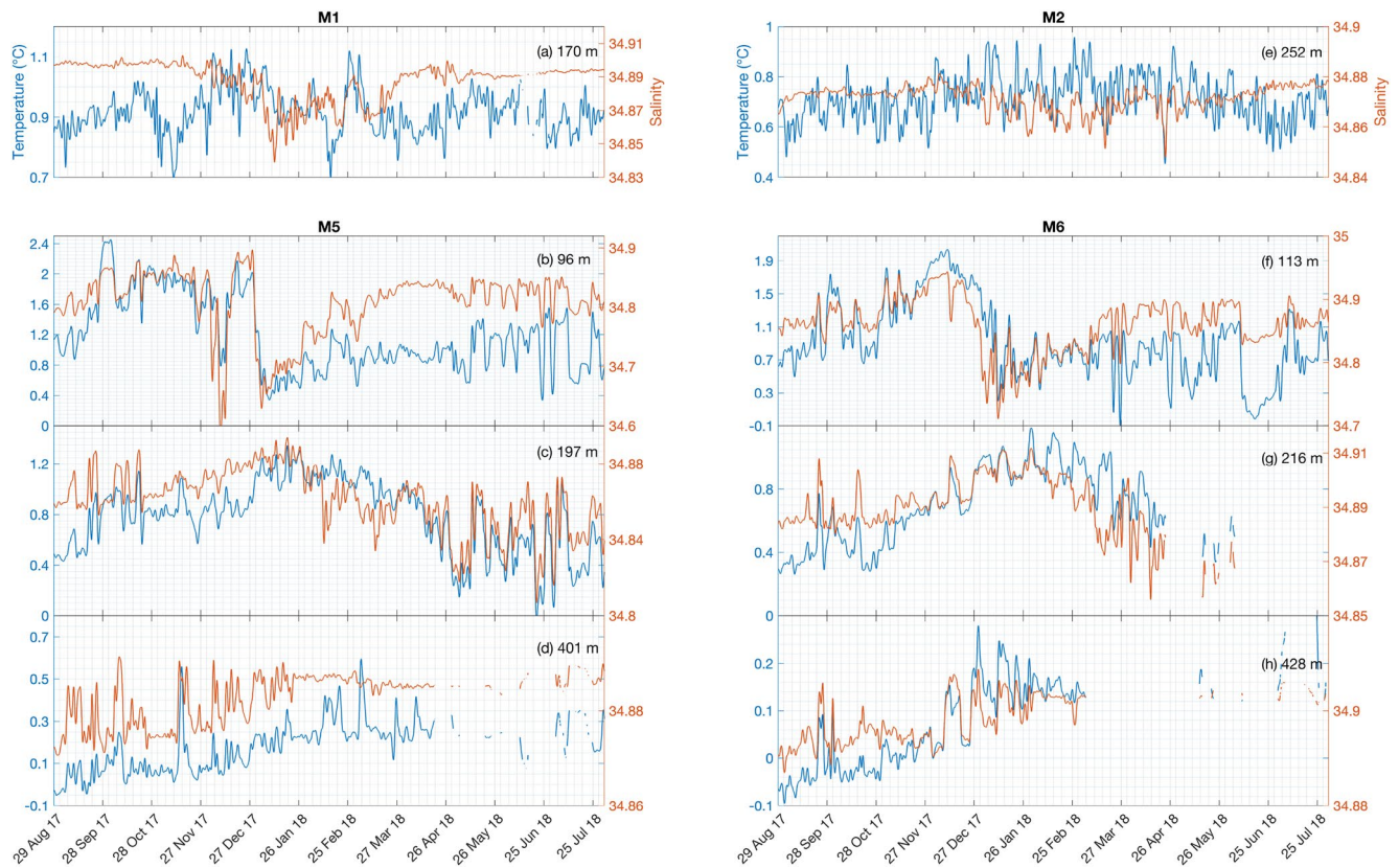
Figure 8. Time series of (blue) temperature and (orange) salinity recorded at (a) M1, (e) M2, (b–d) M5 and (f–h) M6. The depth of the sensor is displayed in the right upper corner.
