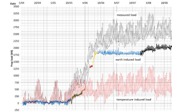
Figure 5. Comparison between the measured load by the strain gauges and the separated earth and temperature-induced loads for prop B1-9
