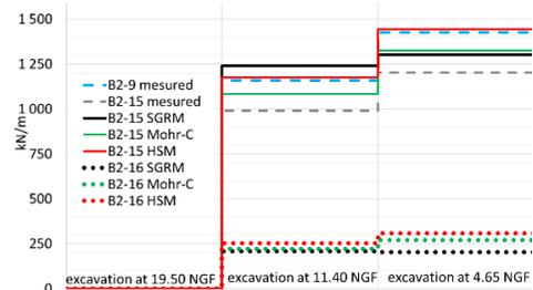
Figure 12. Forces in props at 19.1 and 20.50NGF
